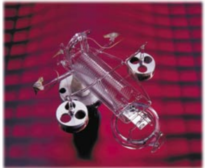
Series 7250's feature Ruska's unique fused-quartz sensor. This rugged transducer offers unequalled precision and a stability of 0.0075% of reading per year.
