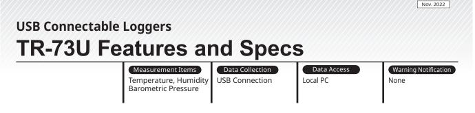
The TR-73U is a three-channel data logger designed to simultaneously measure and record barometric pressure, temperature and humidity.
